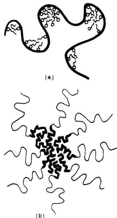
Figure 2. Micellar structures involving polymers: (a) polymer surfactant cluster; (b) self-assembly of a diblock polymer.
